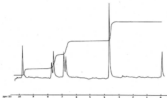
Figure 4. NMR spectrum of C_8H_8O_2 (no peaks removed by D_2O ).
